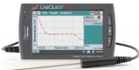
A real-time temperature vs. time graph produced with LQ2 and temp. probe
